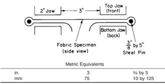
FIG. 1 Illustration of Specimen Placement for Strong Fabrics
