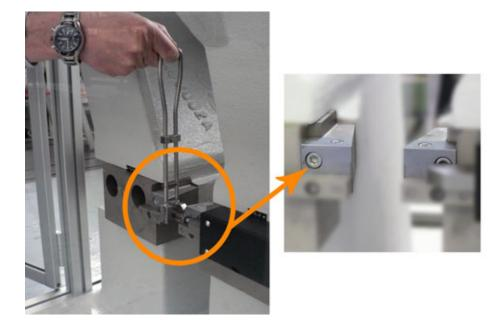
TIA2.3.2 750 J Test supports Charpy according to UNI EN ISO 148-2 and ASTM-E-23 Standard
