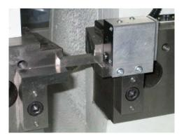
TIA2.8.2 Automatic specimen centering device, on sample V notch, automatically activated at door opening/closing
